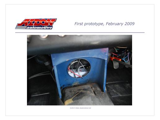
... so we did! This is the first Amethyst prototype, installed in our MGB. This served for approximately two years, and covered some 15,000 miles. It used the Newtronic (aka Piranha) pickup that came with the car, and the Newtronic amplifier, and intercepted and adjusted the signal between the two. Note the vacuum pipe coming from the inlet manifold.
