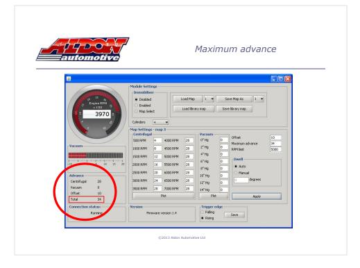
Here we see the maximum advance of 34 degrees being applied, even though the sum of centrifugal advance (28) plus offset (10) exceeds this figure.
