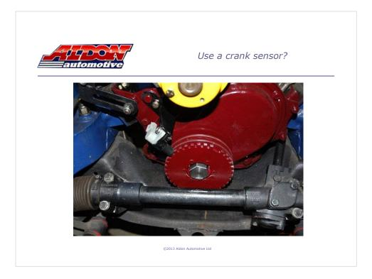
We wanted to replace the centrifugal and vacuum advance mechanisms with a system more similar to the ones used on modern cars. Retrofit mapped ignition systems have been available for several years, but generally use a crank sensor. This is the most accurate way of measuring crank position, but fitting involves a great deal of work (engine out?) and does not look at all original.
