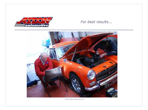
A rolling road session allows best results to be obtained under controlled conditions. Normally, we start with the factory timing characteristic, and advance or retard it to optimise power output. Then, we adjust the timing at various RPM points to optimise mid-range power and efficiency.
