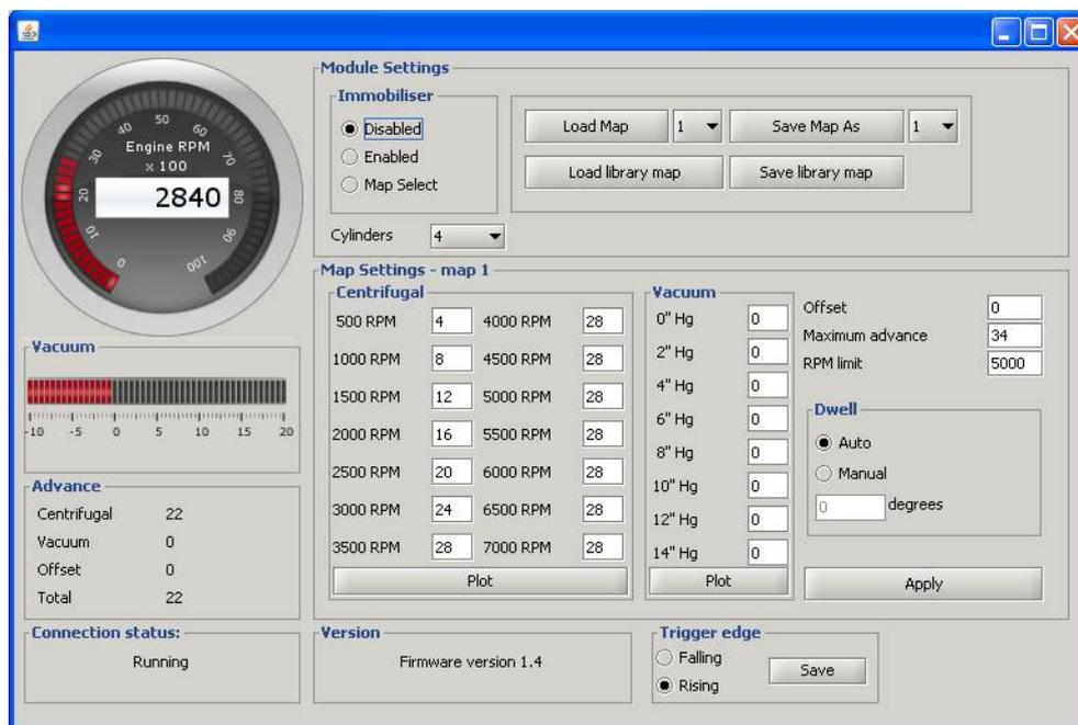
**Note:** The following screen shots were taken using the vacuum version of Amethyst. If you have the boost version, the screen will display pressure from -0.5 to 1.5 bar instead. If you have the TPS version, the screen will display throttle angle, from 0 to 90 degrees.
