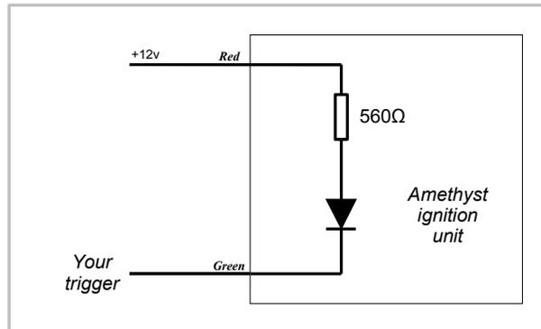
If the circuitry connected to the green wire draws 3mA or more, Amethyst will read this as “points closed”. The input pulse must be of least 50μs duration.
