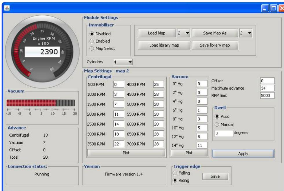
If your Amethyst unit is fitted with a TPS, you will see load points labelled from 0 to 90 degrees, rather than from 0 to 14 inches of mercury. If you have a boost sensor instead of a vacuum sensor, you will see the load points labelled from -0.5 to 1.5 bar.
