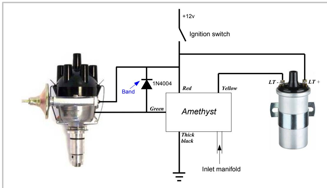
Fig. 5. Using Amethyst with reluctor input
