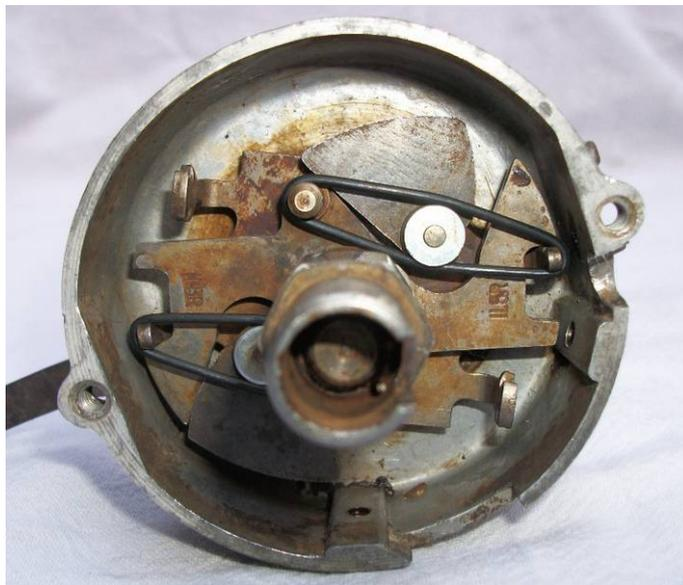
*Fig. 1. Advance mechanism locked using O-rings*
